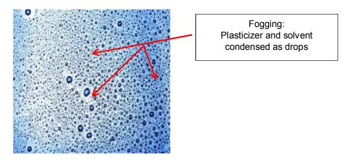
Because of dramatic high volatile and fogging behavior of the cured IG-sealant, the use of the "new Russian polymer" in IG-sealant applications is definitely unsuited. In comparison to that, the volatiles of IG-sealants based on a liquid Polysulfide Polymer, like Thioplast G, are in the range of 0.5% only and mainly based on water out of the IG-sealant formulation (fillers, polymer).
