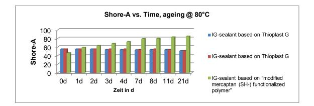
In parallel to the increasing of the Shore A hardness up to Shore D, a significant weight loss up to 3wt% has been noticed.
