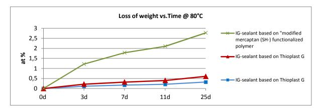
Additionally, a significant loss of elasticity and an increasing of the internal strength (tensile strength) has been found. In contrary, IG-sealants based on Thioplast G are stable in Shore A-hardness and their stress-strain characteristic even after ageing at 80°C.
