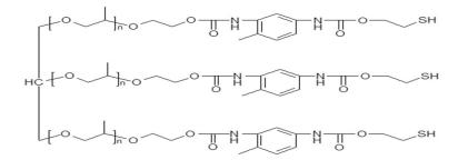
That polymer structure is chemically likely to a Polyether based Polyurethane, what is commonly used in low budget 1-part construction sealant and far from the polymer backbone of a liquid Polysulfide Polymer, well known under the product label "Thioplast G".
